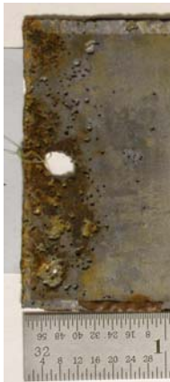
Figure 2: Al409 with corrosion removed.
