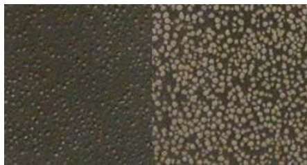
Figure 4: Neukote™ sample - pimples after test completion on the left and pimples removed on the right (approx. 7x).
