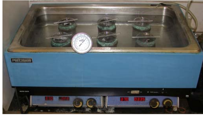
Figure 1: Water Bath Configuration for Performing the J&L Modified Kawasaki Condensate Corrosion test.
